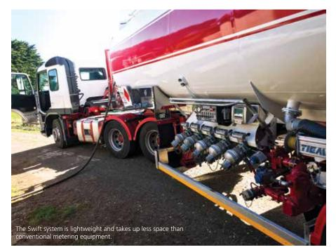
can also preset volumes for gravity, bulk and hose reel discharges.
