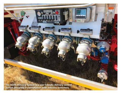
to use, with a simple interface. The core components are those that drivers are familiar with. It's all about level gauging and therefore it doesn't have the flowrate restrictions of a meter. Use of the system is largely based on onscreen prompts that are very straightforward," he says. Liquip Sales Director, Ryan Hawson adds, "When the engineers designed the system, they had a prototype unit out the back and
