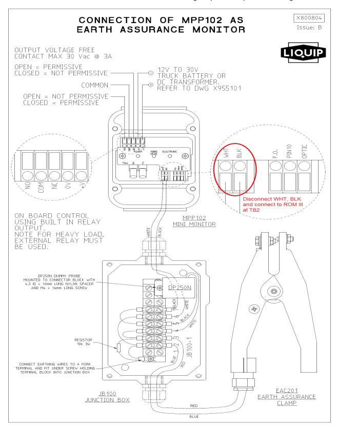
Figure 3. MPP102 configuration for earth assurance
