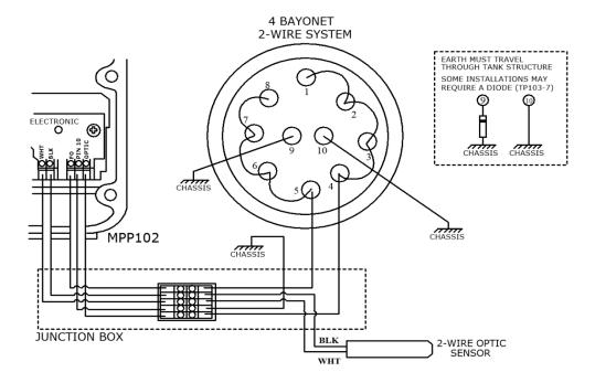
Figure 2a. MPP102 2-wire socket wiring
