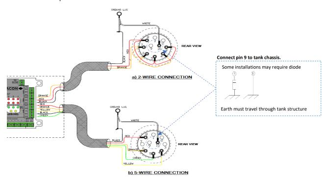
Figure 2b. ROM III socket wiring (2-wire and 5-wire options)
