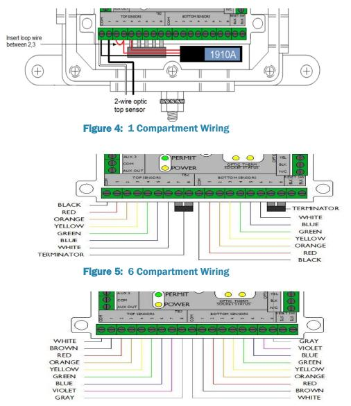
Figure 6: 8 Compartment Wiring
