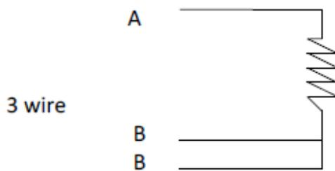
Most common connection 3 wire, the instrument measures the lead wire resistance in the B legs and allows for this in its reading.
