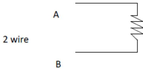
Basic connection where the lead is short. No lead wire compensation, introducing an error into the reading.
