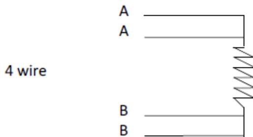
4 wire connection is the most accurate measurement. The instrument measures the lead resistance of all four lead wires removing these values for its reading
