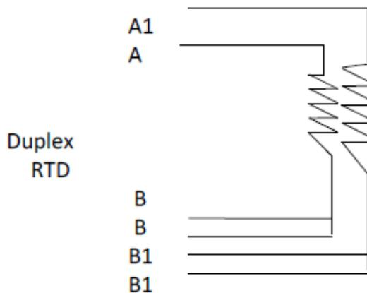
Duplex 3 wire RTD connection as per single RTD but two individual element windings.
