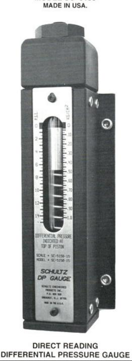
Schultz Engineered Products Model SC-5150 Direct Reading piston type differential pressure indicator is designed to accurately and reliability read differential pressure across filter vessels. The gauge consists of a spring corrosion resistant piston moving inside an annealed glass cylinder. Differential pressure is easily read from the top of the piston.
