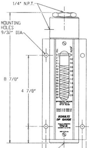
If gauge is used for Av gas use option A this provides on ultraviolet shield to prevent accumulation of fuel dye inside cylinder (there is no charge at time of purchase).
